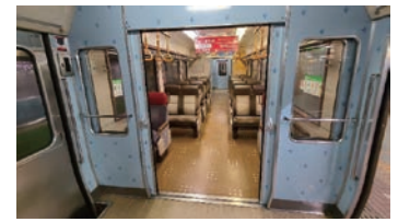
Ventilating by opening the partition doors between train cars
