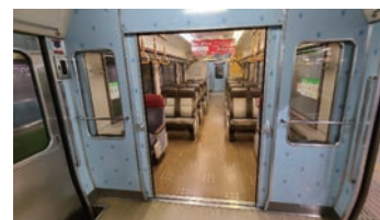
Ventilating by opening the partition doors between train cars
