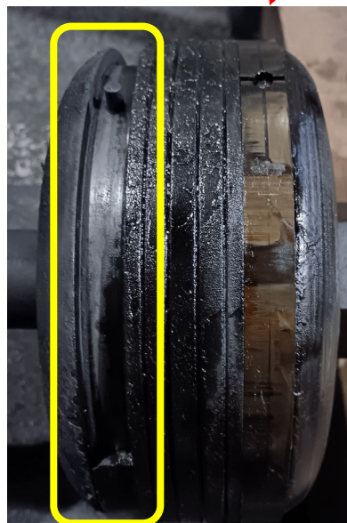
Damaged piston ring (area outlined in yellow)
